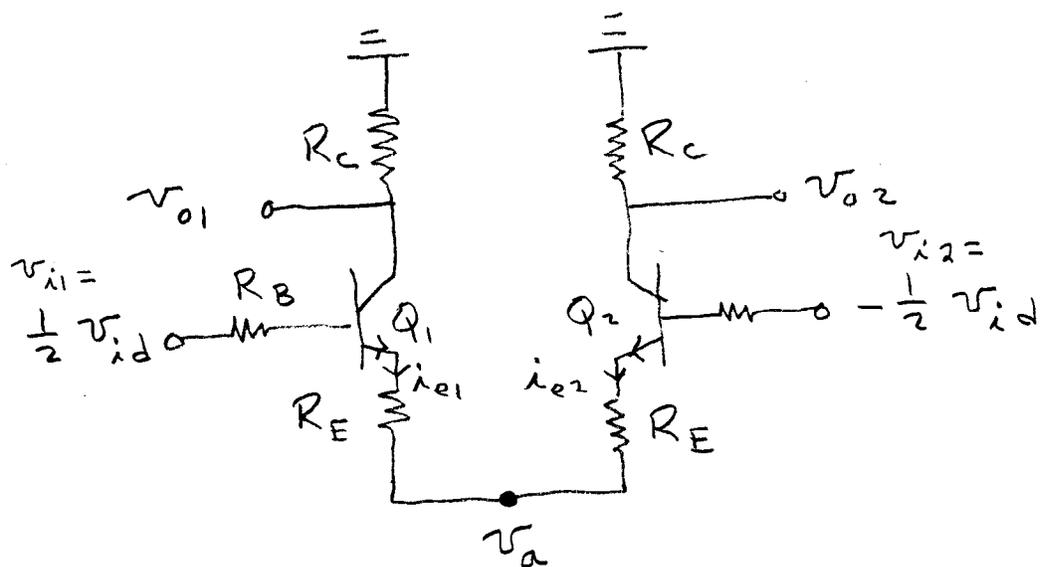
$v_{i1}$  forces  $v_a$  to increase while  $v_{i2}$  forces  $v_a$  to decrease. The net effect is  $v_a = 0$ . Thus we obtain the equivalent circuit.
