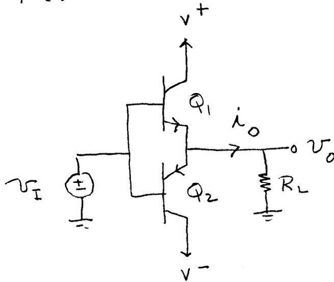
This stage is commonly used as the output stage in an op amp. It acts as a buffer stage.  $Q_1$  supplies positive  $i_O$  and  $Q_2$  supplies negative  $i_O$ .
