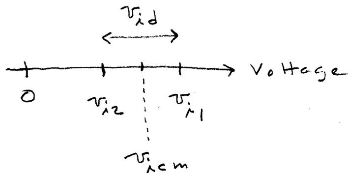
We can use superposition of  $v_{id}$  and  $v_{icm}$  to solve for  $v_{o1}$  and  $v_{o2}$ .
