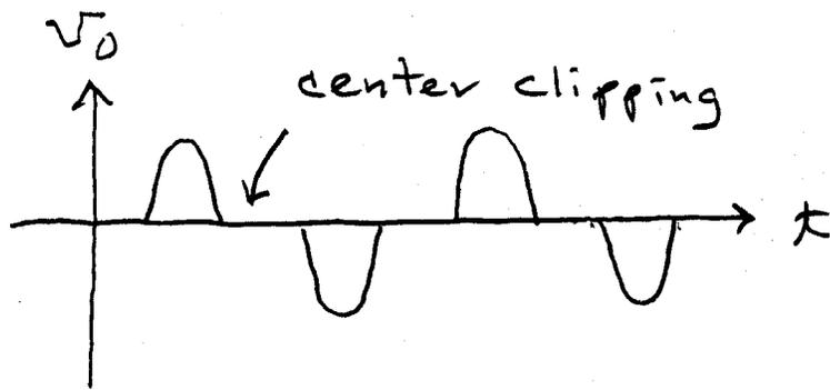
To minimize the center clipping,  $Q_1$  and  $Q_2$  must be biased on when  $v_I = 0$ . A possible circuit is
