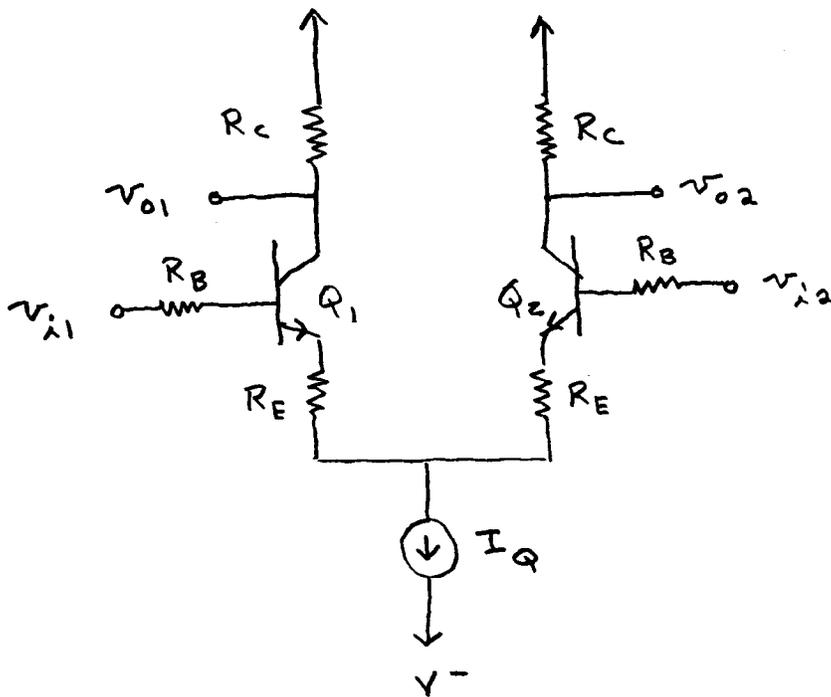
For the dc bias solution, set  $v_{i1} = v_{i2} = 0$ . If the BJTs are identical,  $I_Q$  splits equally between  $Q_1$  and  $Q_2$ .
