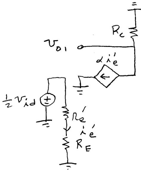
$$i_e' = \frac{1}{2} v_{id} \frac{1}{r_e' + R_E}$$
