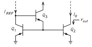
4. The figure shows a Wilson current mirror (a) If the transistors are identical and the Early effect can be neglected, label all currents in the unlabeled branches in terms of  $I_O$ . Hint, express  $I_{E3}$  in terms of  $I_O$  and use the results of problem 2 to show that  $I_{C1}$  is given by n terms of  $I_{E3}$
