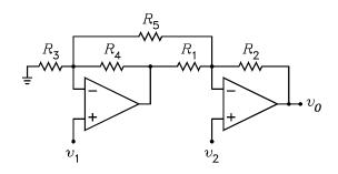
19. For  $R_1 = 10 \text{ k}\Omega$ ,  $R_2 = 30 \text{ k}\Omega$ ,  $R_3 = 20 \text{ k}\Omega$ , and  $V_1 = 4 \text{ V}$ , show that  $v_O = 10 \text{ V}$ . Hint: The answer is independent of  $R_1$ .
