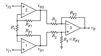
15. The figure shows a balanced output amplifier. Design the circuit so that  $v_{O1} = -v_{O2} = 6v_I$ . When  $v_{O1} = \pm 12$  V and  $v_{O2} = \mp 12$  V, the current through  $R_{F1}$  and  $R_{F2}$  is not to exceed 1 mA. Answers: for 1 mA,  $R_1 = 2$  k $\Omega$ ,  $R_{F1} = 10$  k $\Omega$ , and  $R_{F2} = 12$  k $\Omega$ .
