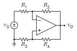
22. For  $I_1 = 1 \text{ mA}$ ,  $R_1 = 3 \text{ k}\Omega$ ,  $R_2 = 4 \text{ k}\Omega$ ,  $R_3 = 2 \text{ k}\Omega$ , and  $R_4 = 1 \text{ k}\Omega$ , show that  $v_O = -1 \text{ V}$ . Hint: Use superposition of  $I_1$  and  $v_O$  to solve for the voltage at the two op-amp inputs. Set the voltages equal to each other to solve for  $v_O$ .
