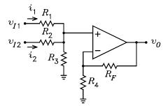
10. Fig. (a) shows a differential amplifier. Fig. (b) shows the equivalent circuit for the special case  $R_1 = R_3$  and  $R_2 = R_F$ . It is desired to design the circuit so that  $v_O = 10 (v_{I1} - v_{I2})$ . In addition, the input resistance seen between the two input nodes is to be  $10 \,\mathrm{k\Omega}$ .
