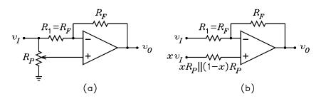
(a) Prove that the Thévenin equivalent circuit seen looking out of the  $v_+$  input is the one shown in Fig. (b). What is the maximum source resistance of this Thévenin circuit? Answer:  $25 \text{ k}\Omega$ .
