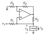
(a) With the load open circuited, i.e.  $i_L = 0$ , use superposition of  $v_1$  and  $v_O$  to show that  $v_{L(oc)} = (v_1R_2 + v_OR_1) / (R_1 + R_2)$ . Show that  $v_O = v_{L(oc)} (1 + R_F/R_3)$ . (a) Solve the equations from the previous part to show that
