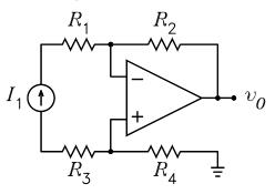
21. For  $R_1 = 50 \,\mathrm{k\Omega}$ ,  $R_2 = 20 \,\mathrm{k\Omega}$ ,  $R_3 = 10 \,\mathrm{k\Omega}$ , and  $R_4 = 40 \,\mathrm{\Omega}$ , show that  $v_O/v_S = 5/9$ .
