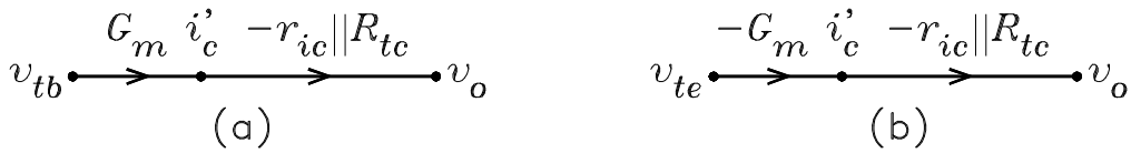
Figure 7: (a) Flow graph for the CE amplifier. (b) Flow graph for the CB amplifier.
