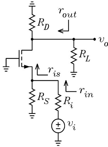
Figure 3: Signal circuit.
