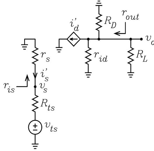
Figure 6: Source equivalent circuit.
