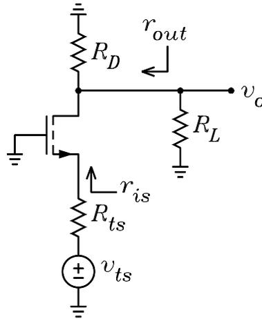
Figure 4: Signal circuit with Thévenin source circuit.
