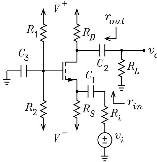
Figure 1: Common-gate amplifier.
