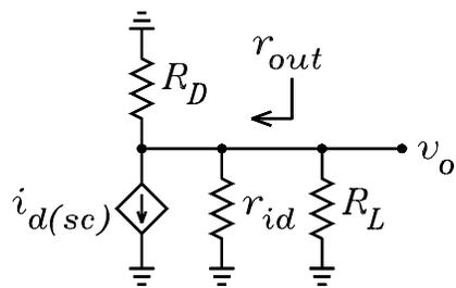
Figure 5: Norton collector circuit.
