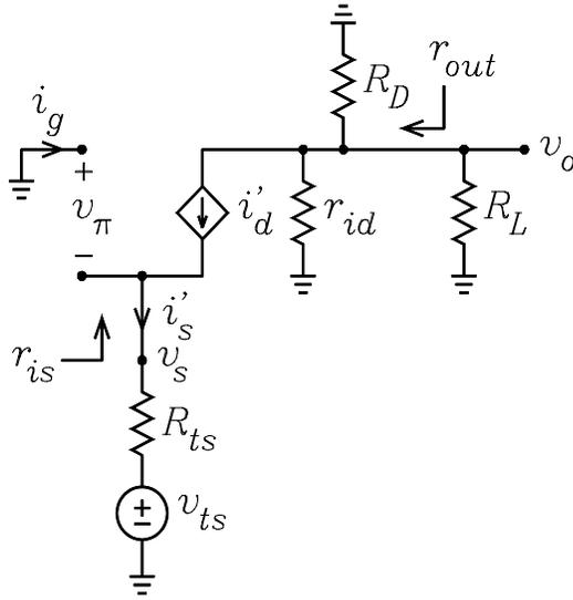
Figure 7: Hybrid  $\pi$  model circuit.
