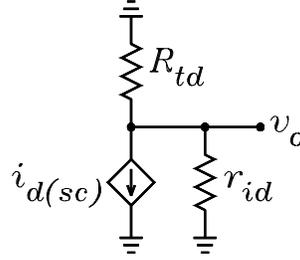
Figure 5: Norton drain circuit.
