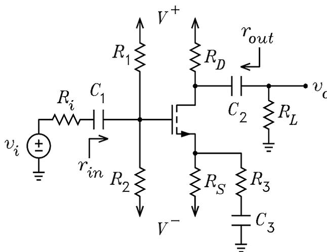
Figure 1: Common-source amplifier.
