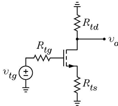
Figure 4: Signal circuit with Thévenin gate circuit.
