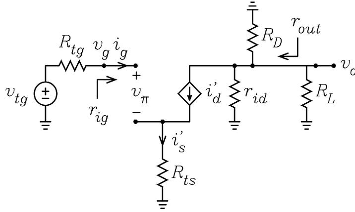
Figure 7: Hybrid  $\pi$  model circuit.
