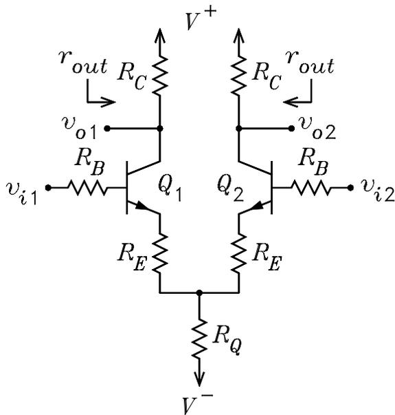
$$V_T := 0.025 \quad r_x := 30 \quad V_p := 24 \quad R_C := 24000 \quad \beta := 74 \quad \alpha := \frac{\beta}{1 + \beta} \quad \alpha = 0.987$$
