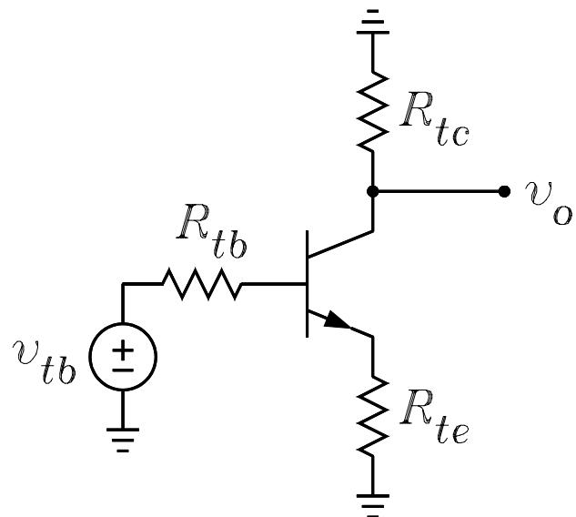
$$v_{tb} := v_s \cdot \frac{R_P(R_1, R_2)}{R_S + R_P(R_1, R_2)} \quad v_{tb} = 0.916$$
