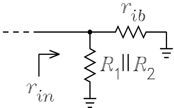
$$r_{ib} := r_x + (1 + \beta) \cdot (r_e + R_P(R_{te}, r_0 + R_{tc})) - \frac{\beta \cdot R_{te} \cdot R_{tc}}{R_{tc} + r_0 + R_{te}}$$
