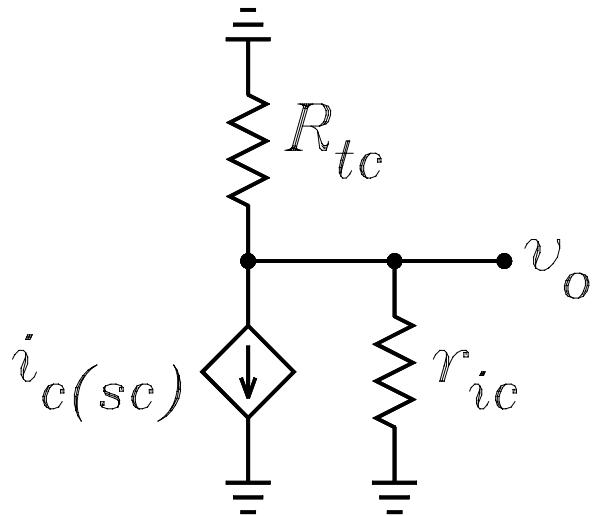
$$r_{ic} := \frac{r_0 + R_P(r'_e, R_{te})}{1 - \frac{\alpha \cdot R_{te}}{r'_e + R_{te}}} \quad r_{ic} = 1.3577 \cdot 10^5$$
