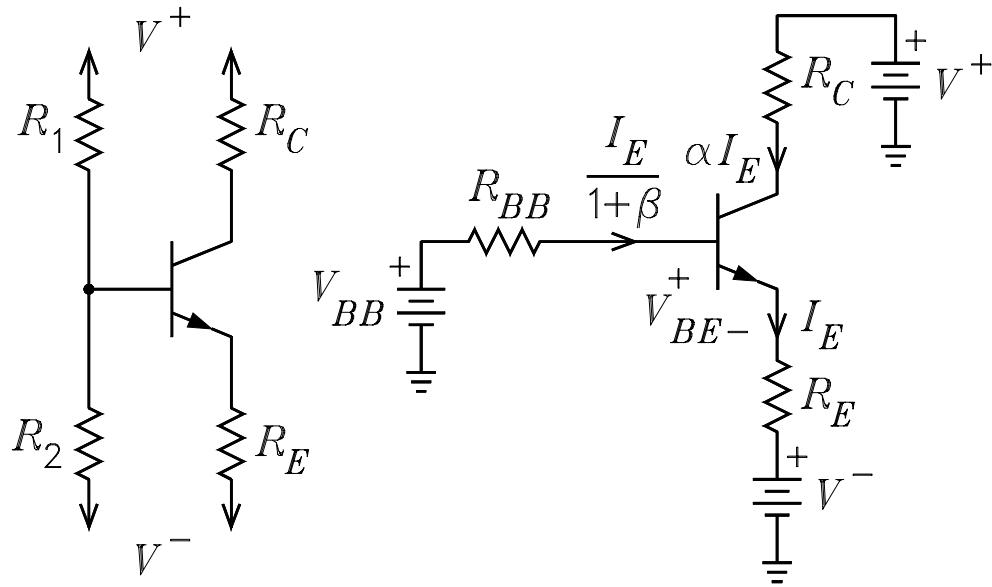
$$V_{BB} := \frac{V_p \cdot R_2 + V_m \cdot R_1}{R_1 + R_2} \quad V_{BB} = 1.3636$$
