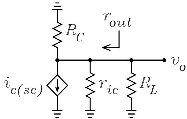
$$r_{out} := R_P(R_C, r_{ic}) \quad r_{out} = 4.168 \cdot 10^3$$
