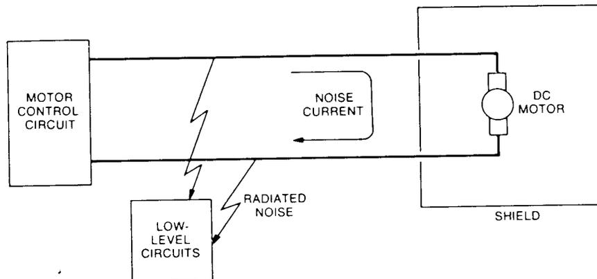
**Figure 1-12.** In this example the noise source is the motor, and the receptor is the low-level circuit. The coupling channel consists of conduction on the motor supply leads and radiation from the leads.
