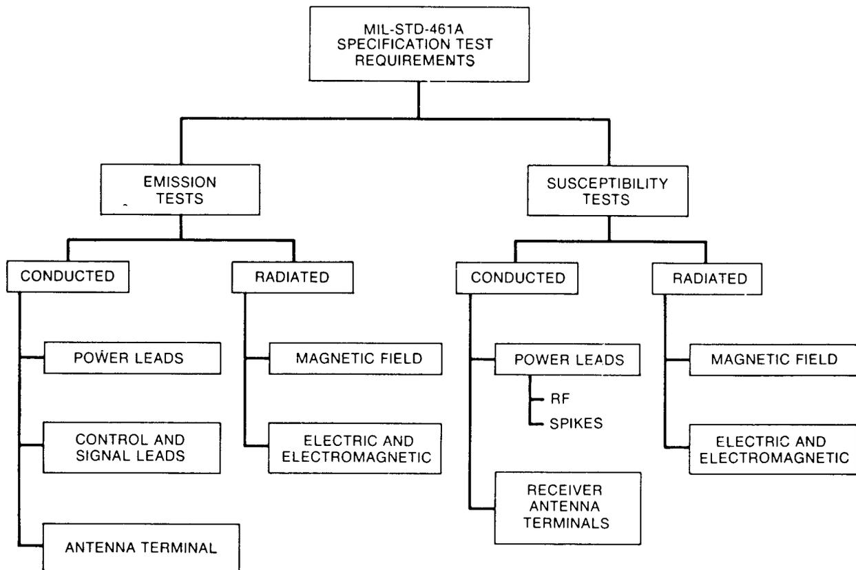
**Figure 1-10.** Military specifications cover both the emission of noise and the susceptibility to it. In both cases tests of conducted and radiated noise are specified.
