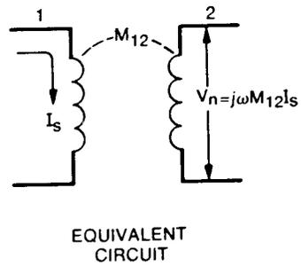
**Figure 1-14.** When two circuits are coupled by a magnetic field, the coupling can be represented as a mutual inductance.
