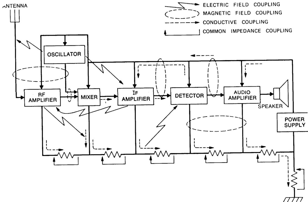
**Figure 1-1.** Within equipment, such as this radio receiver, individual circuit elements can interfere with one another in several ways.
