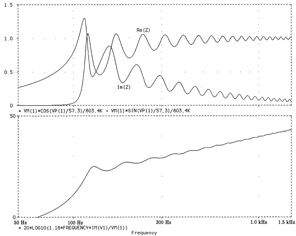
FIG. 6. (Upper) Real and imaginary parts of throat acoustic impedance for example horn B. (Lower) Magnitude of normalized pressure transfer function in dB for horn B.
