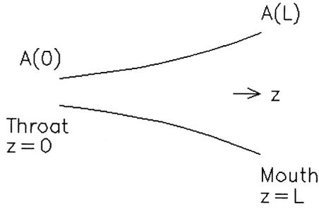
FIG. 1. Schematic drawing of acoustic horn of length  $L$ .
