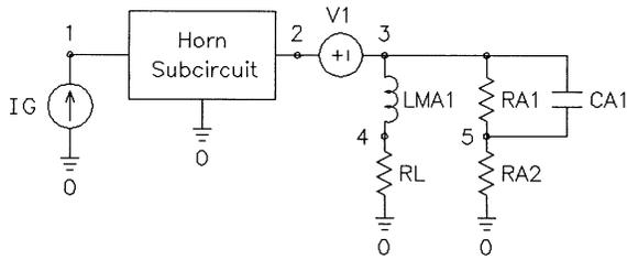
FIG. 4. Circuit used to calculate throat acoustic impedance of example horns.
