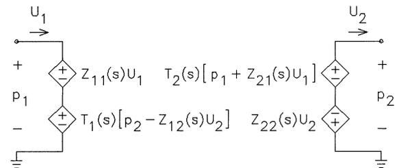
FIG. 2. Controlled-source analogous circuit for horn.
