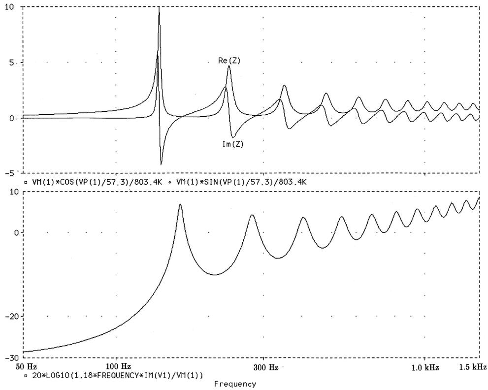
FIG. 5. (Upper) Real and imaginary parts of throat acoustic impedance for example horn A. (Lower) Magnitude of normalized pressure transfer function in dB for horn A.
