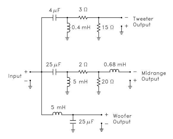
Resistors are 10 watt or greater. Capacitors should have a voltage rating of 100 volts or greater. Inductors are air core wound with 18 gauge wire. Note that the midrange and tweeter are connected with the + or "red dot" connected to the ground output.
