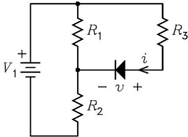
$$V_S = V_1 \frac{R_1}{R_1 + R_2} = 10\text{ V} \quad R_S = R_1 \parallel R_2 + R_3 = 2\text{ k}\Omega$$
