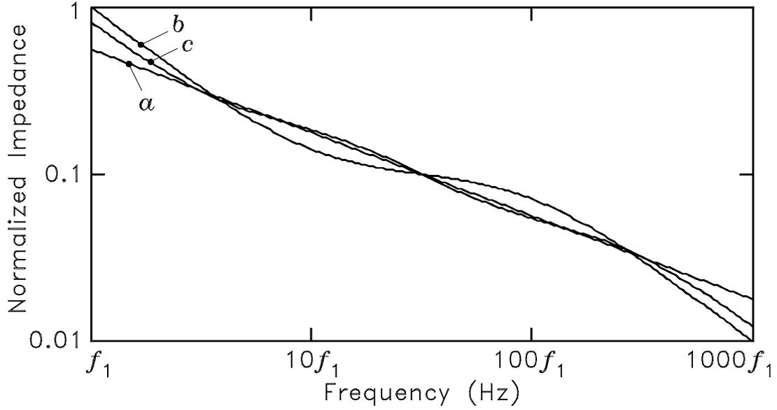
Figure 2: Example plots of the desired impedance (curve *a*) and the approximating impedances (curves *b* and *c*) versus frequency for the case  $n = 0.5$ .
