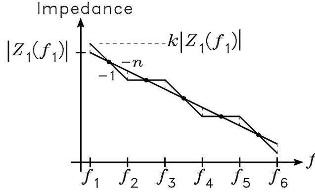
Figure 1: Magnitude plots of the desired impedance and the asymptotes of the approximating impedance versus frequency.
