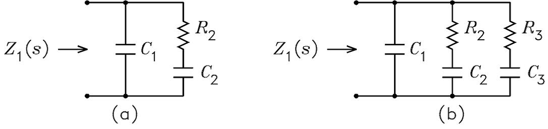
Figure 3: Circuits for approximating the impedance  $Z_1(j\omega)$ .
