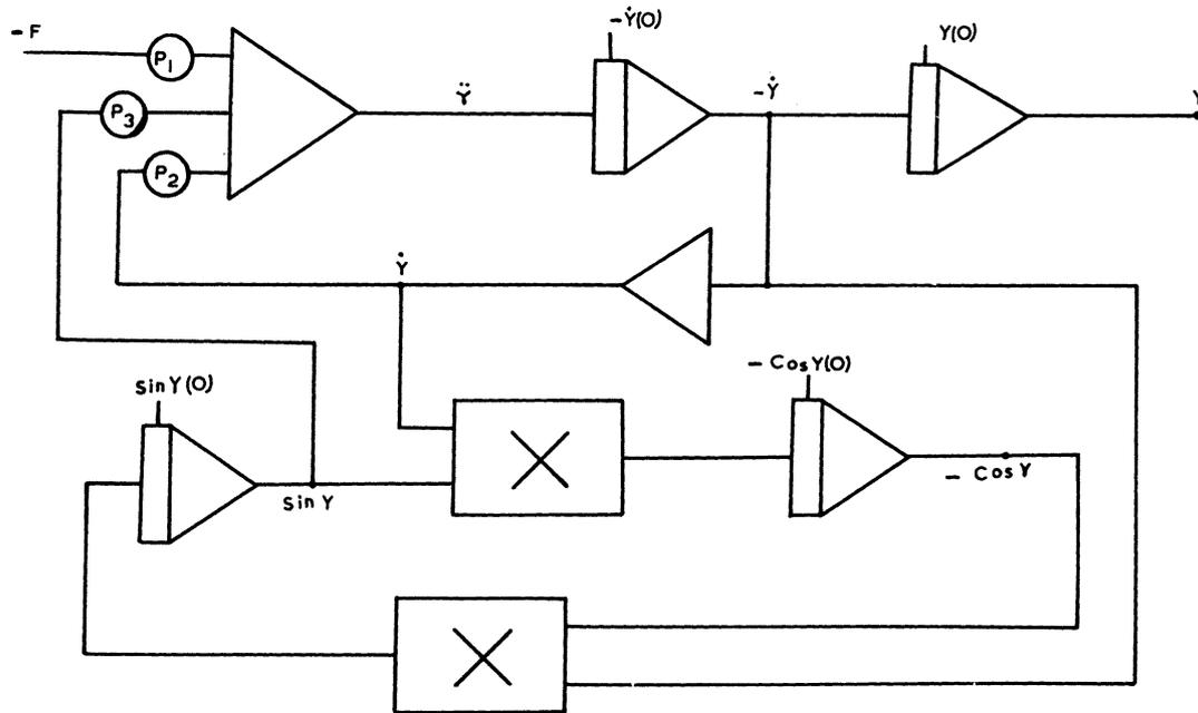
Fig. 4. Computer circuit for solving the nonlinear differential equation  $\ddot{y} + c\dot{y} + k(\sin y) = F$ . Potentiometer settings:  $P_1 = 1.0$ ;  $P_2 = c$ ;  $P_3 = k$ .
