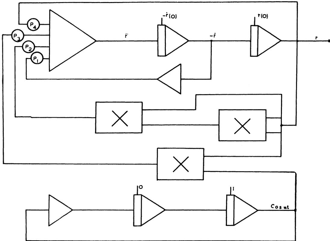
Fig. 5. Computer circuit for simulating Melde's system. Potentiometer settings:  $P_1=c$ ;  $P_2=b$ ;  $P_3=1.0$ ;  $P_4=a$ .
