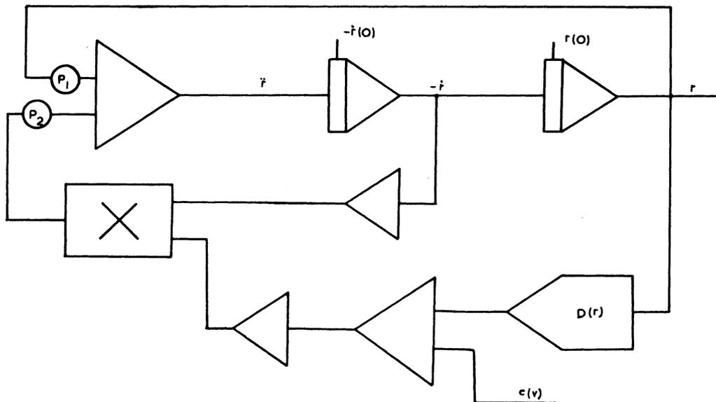
Fig. 6. Computer circuit for studying the oscillations of a suspension bridge. Potentiometer settings:  $P_1=a$ ;  $P_2=1.0$ .
