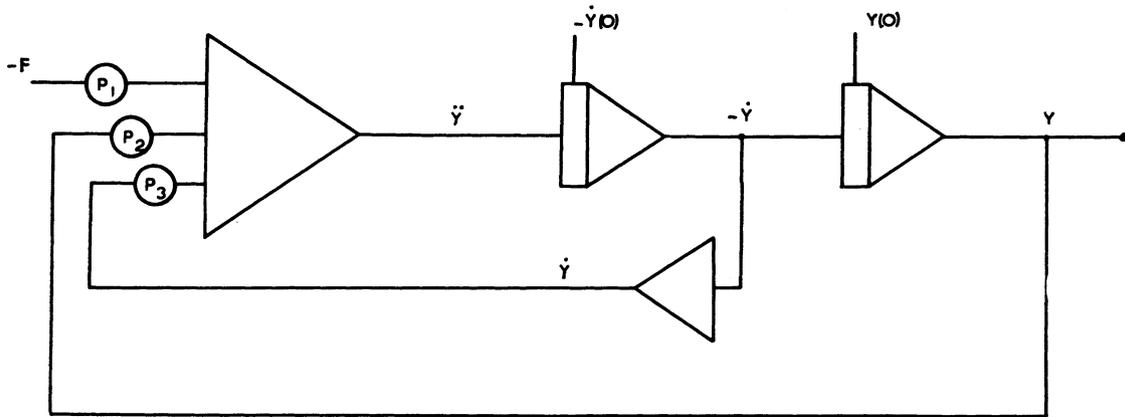
Fig. 2. Computer circuit for solving the equation  $m\ddot{y} + n\dot{y} + ky = F$ . Potentiometer settings:  $P_1 = 1/m$ ;  $P_2 = k/m$ ;  $P_3 = n/m$ .
