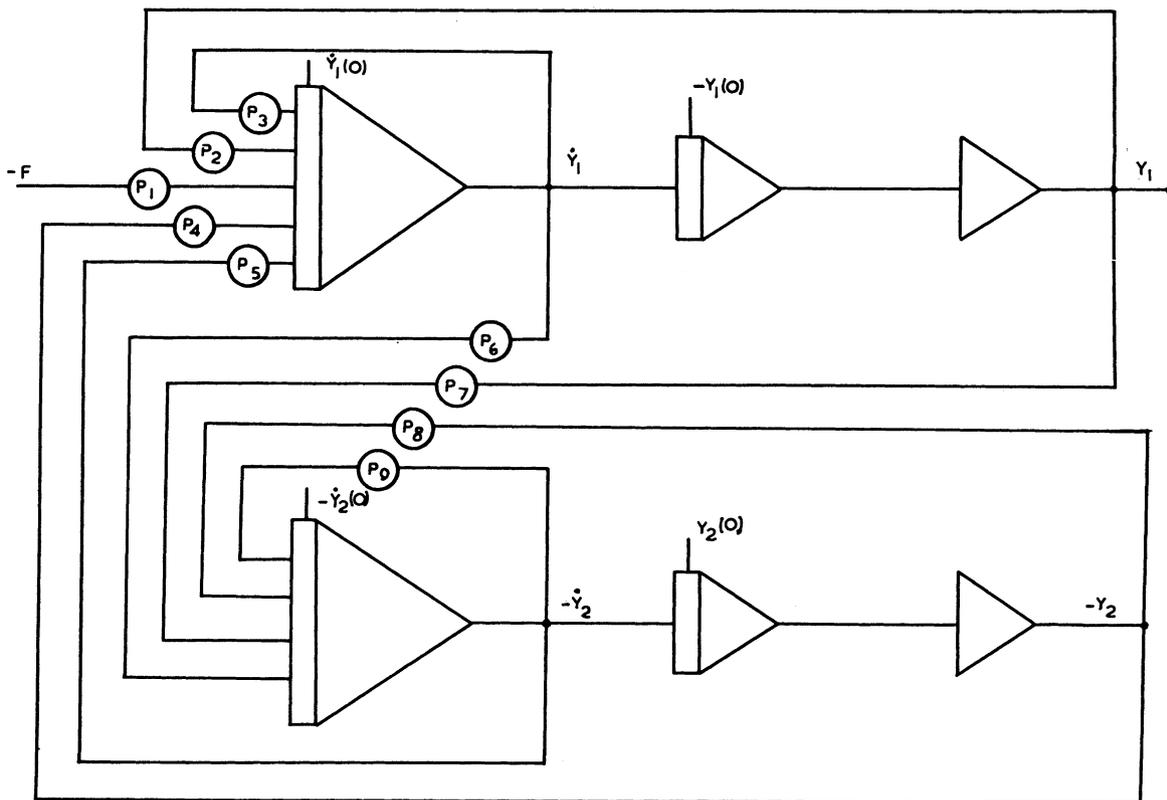
Fig. 3. Computer circuit for solving the simultaneous differential equations given in (3). Potentiometer settings:  $P_1 = 1/m_1$ ;  $P_2 = k_1/m_1$ ;  $P_3 = n_1/m_1$ ;  $P_4 = b_2/m_1$ ;  $P_5 = a_2/m_1$ ;  $P_6 = a_1/m_2$ ;  $P_7 = b_1/m_2$ ;  $P_8 = k_2/m_2$ ;  $P_9 = n_2/m_2$ .
