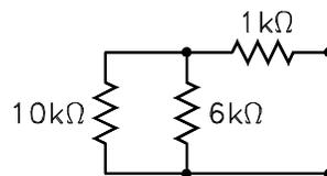
6. Calculate the spot noise voltage at the output of the circuit at the frequency  $f = 1.5$  kHz. Assume  $T = T_0 = 290$  K. [9.83 nV/ $\sqrt{\text{Hz}}$ ]
