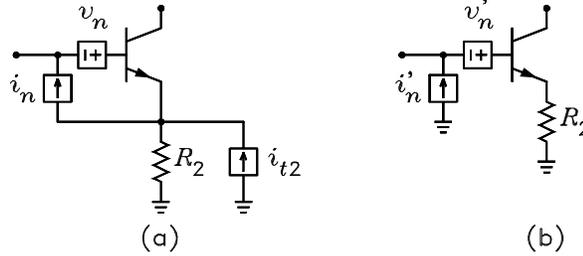
4. The figure shows the ac signal circuits for single stage CE and CB amplifiers. The transistor parameters are  $\beta = 100$ ,  $r_x = 40 \Omega$ ,  $r_0 = 50 \text{ k}\Omega$ , and  $V_T = 25 \text{ mV}$ . (The equations for the voltage gain, input resistance, and output resistance of the CE and CB amplifiers are given in Section 7.6 of the class notes. You do not have to derive these.)
