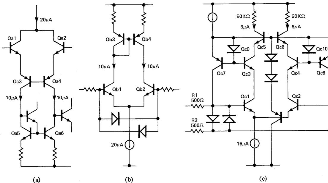
Fig. 4. Three op amp input stages. (a) 741-active load. (b) n-p-n input-active load. (c) Resistive load with bias current cancellation.
