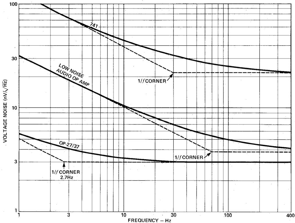
Fig. 2. Noise spectra of three operational amplifiers.
