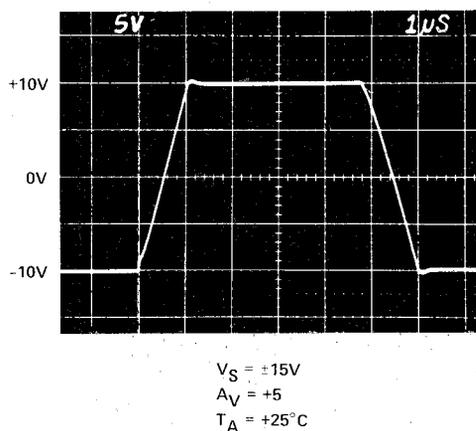
Fig. 12. Large signal transient response.
