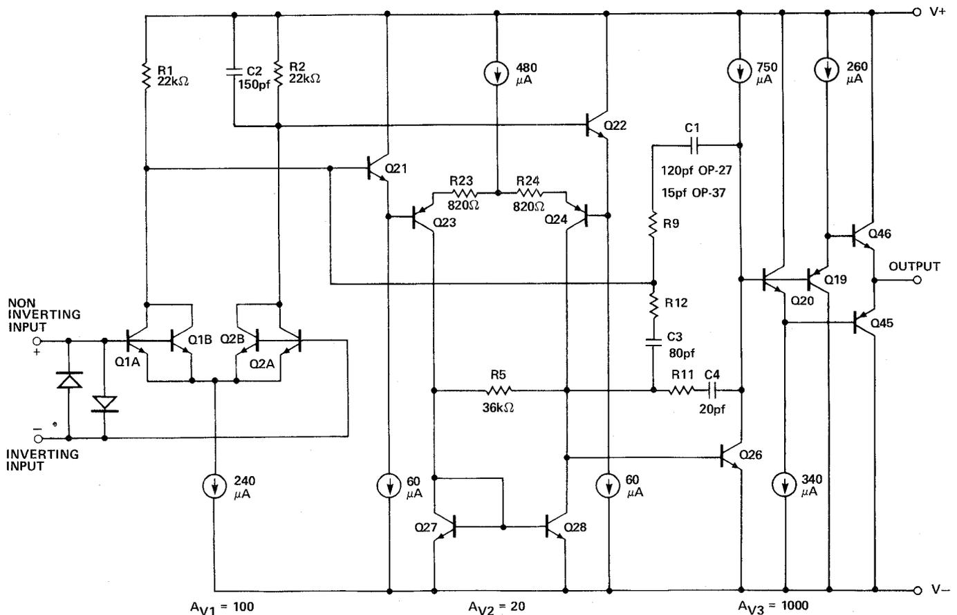
Fig. 7. Low noise op amp simplified schematic.
