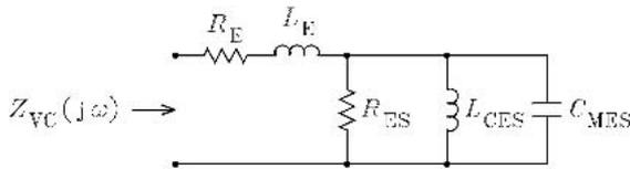
Fig. 1. Equivalent circuit of voice-coil impedance.
