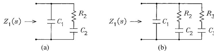
Fig. 5. Circuits for approximating impedance  $Z_1(j\omega)$ .
