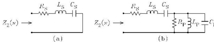
Fig. 6. Compensation circuits for low-frequency impedance rise. (a) Infinite-baffle and closed-box drivers. (b) Vented-box drivers.
