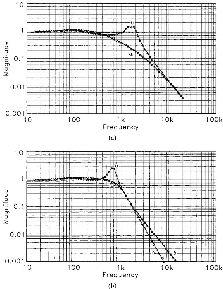
Fig. 10. Voice-coil voltage of JBL driver with (curve a) and without (curve b) Zobel network A. (a) Second-order crossover network. (b) Third-order crossover network.
